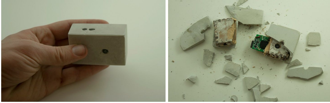
An Inaccessible Digital Camera with a concrete enclosure.
