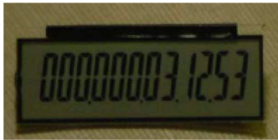
Figure 2. The Lamp that Counts displays the total number of years, days, hours, minutes, seconds and milliseconds the lamp has been lit during its lifetime (milliseconds not shown in this prototype).
