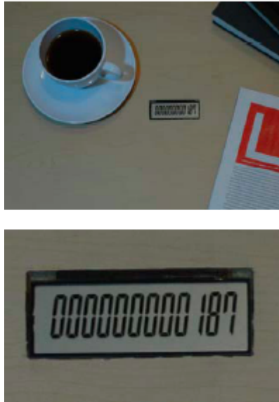
Figure 1. The Table that Counts displays the total number of heavy objects that have been placed on it during its lifetime.
