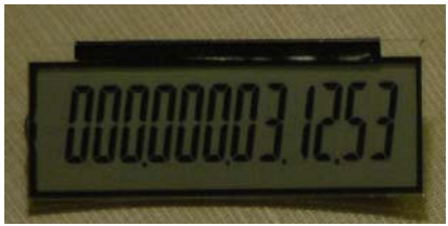
Figure 2. Lamp that Counts displays the total number of years, days, hours, minutes, seconds and milliseconds the lamp has been lit during its lifetime (milliseconds not shown in this prototype).
