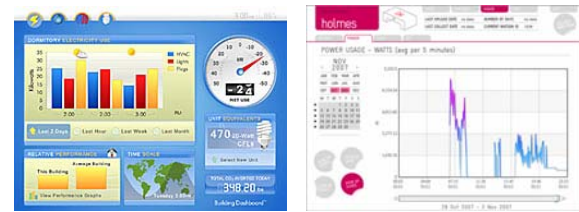
Figure 2. Lucid Building Dashboard (left) [Brun, (2008)] and Holmes [DIY Kyoto, (2008)] (right) allow dwellers to explore in detail the patterns of consumption within their home or building.
