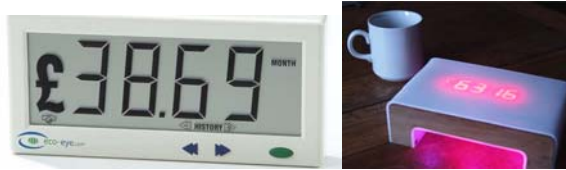
Figure 3. The Eco-Eye [Eco-Eye.com, (2008)] (left) provides direct feedback on household electrical consumption, while the Wattson [DIY Kyoto, (2008)] (right) additionally provides ambient feedback.
